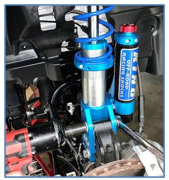
22. Attach ABS line to the left shock – Slide ABS line holder onto tab on back side of shock until it clips in.
