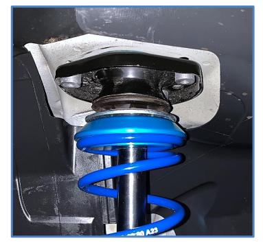
20. Reuse the factory upper mount plate inside the cab and the factory bolts to attach the upper mount. Install bolts and tighten to factory specs. When you are finished tightening upper mounts, replace tool tray, floor mats and trim pieces.
