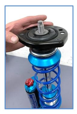
14. Place the upper washer on top of the upper mount with the flat side facing down.
