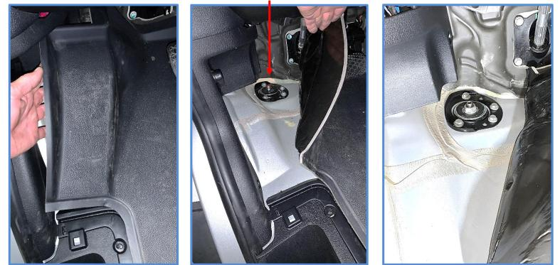
6. Remove upper mounting bolts using a 13mm socket. Save hardware, you will reuse hardware and steel plate to install King shocks.
