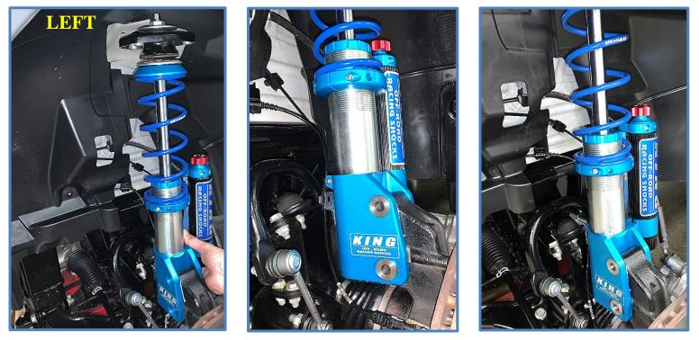
18. Make sure the steel inserts are in place and install the factory bolts through the lower mount. Thread nuts on but do not tighten yet.
