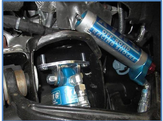
3. Place the reservoir mount onto the studs on top of the factory shock mount. Place the supplied 10mm washer on the stud followed by the 10mm nut provided in the kit. Tighten nuts to 35 ft lbs.
