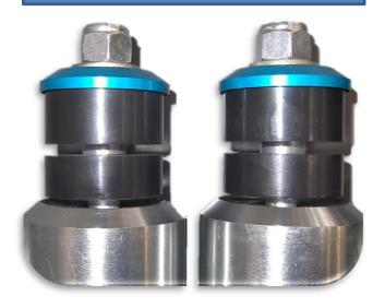
3. For the lower mount place one spacer on the mounting stud (A), then install the rod end followed by the other spacer. Make sure that the spacer is not sitting past the mounting stud (B). Use the factory bolt and tighten to factory specs (C). See photos on next page for proper shock orientation, position shocks accordingly and tighten the nut on the upper mount.
