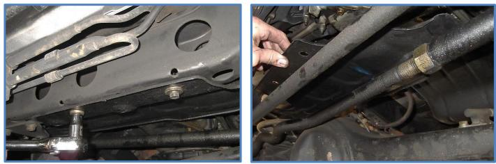
2. Remove the nuts on both ends of the factory steering stabilizer using a 17mm socket/wrench. You may need a ball joint tool or pickle fork to separate the tapered ends from the mounts.
