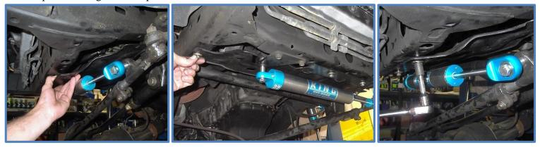
Double check your install, make sure the stabilizer is mounted properly and all hardware is tight. Recheck the hardware after 50 miles and periodically after that as part of routine maintenance.
