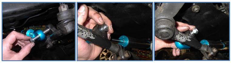
4. Install cylinder end to the factory mount on the opposite side. Insert the tapered spacer into the factory mount. Install the provided 10mm hardware as shown and tighten nut to 50 ft/lbs.
