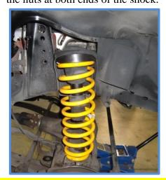
2. Install King Shocks. Be aware that the shocks are side specific. Also be aware that the bushings are different thicknesses, the thicker bushings should be facing toward the cylinder. Install shocks with the thick bushing on the cylinder side of the mounts and the thinner bushing on the end of the shock with the anodized washer, flat washer and lock nut as shown in the photos below. Do not tighten yet, just get the nuts started to hold shock in place.
