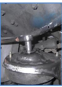
4. Place the reservoir in the side specific reservoir bracket so the hose is behind the bracket. Then position the bracket on the studs on top of the coil bucket.
