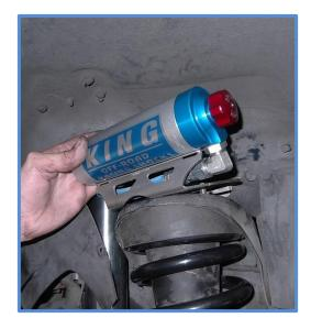
5. Install the nuts that were removed back on the studs and tighten. On the driver's side reinstall the steering shaft guard. Center the reservoir in the cradle and position the shock accordingly so that your install looks like the photo below.
