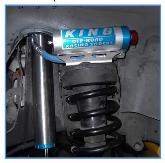
6. Install the provided hose clamps and tighten.
