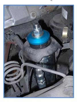
8. For the lower mount use a 10mm wrench to hold the stud to keep the shaft from spinning while tightening.
