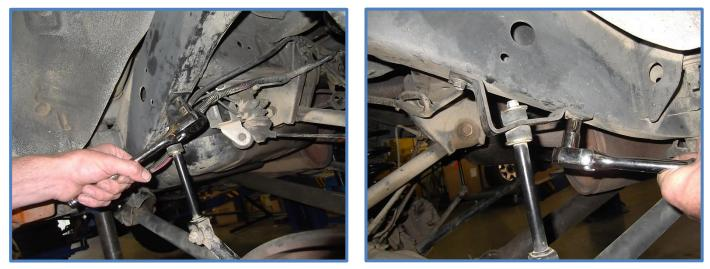
3. Place brackets in position on the frame lined up with the sway bar mounting holes. Brackets are side specific, be sure to mount brackets on the proper side (see photos below - Photos show right side being installed). Use the OE bolts you just removed to bolt the sway bar bracket back in place over the reservoir bracket.
