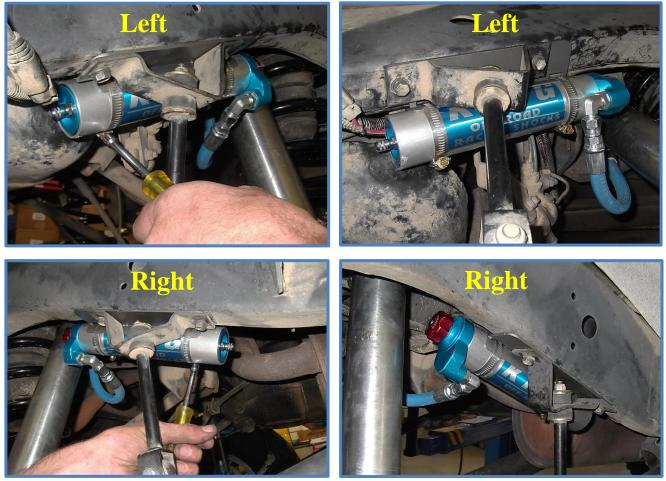
9. Tighten upper mounting pin nuts. Make sure the hose makes a nice loop to the reservoir, adjust shock and reservoir accordingly. Tighten the upper nuts using a 3/4 socket/wrench.
