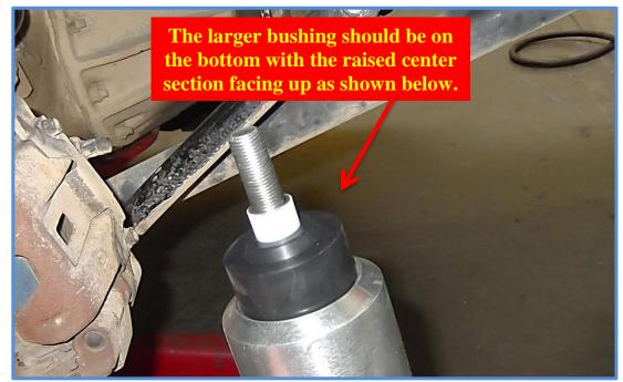
5. Place the shock in the upper mount and install the upper bushing with the blue anodized washer, regular washer and nut. Thread the nut onto the stud but don't tighten yet.
