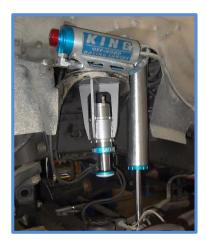
7. Install springs - Unbolt the lower shock mounts, lower the axle enough to install coil springs. Place springs over the bump stop bracket and align with the lower spring perch on axle. Jack axle back up so you can reinstall the lower shock mount hardware. Tighten lower shock mount nuts.
