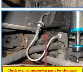
check over all suspension parts for clearance issues. Also check axle/third member for clearance issues with engine, oil pan etc....
