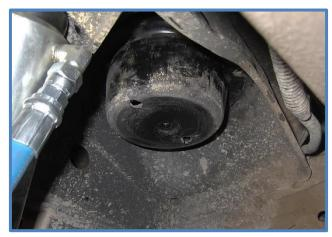
3. Using a 2 ½" hole saw, cut a hole in the center of the bump stop mount using the threaded hole in the center as a guide for the pilot bit.
