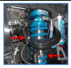
10. Install the sway bar to the threaded holes in the reservoir bracket using the 3/8 x 3/4" bolts and washers provided in the kit. The factory sway bar brackets are side specific and stamped "L" and "R" with an arrow that points toward the front of the vehicle. After the sway bar is mounted to the frame you can reconnect the sway bar links to the steering knuckle.
