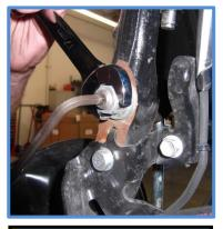
Use an allen wrench to hold the sway bar link stud for removing and tightening nut.
