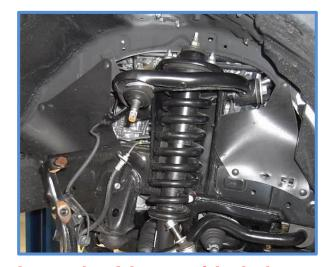
For Lexus GX470 you will need to remove and unplug the control module on top of the shock.
