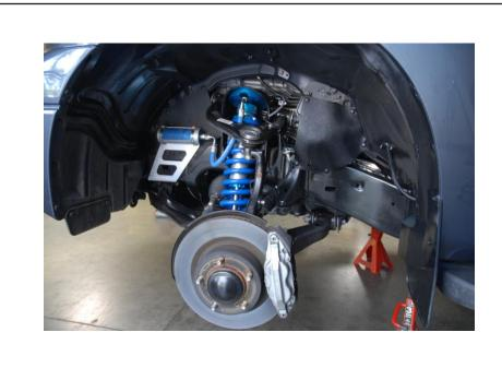
Reconnect A-arms, sway bar links and brake line brackets. Install the reservoir in the reservoir bracket using the supplied hose clamps. Make sure the reservoir hose is routed as shown and does not rub on the moving parts of the suspension. Reinstall the skid plate and check to make sure all your bolts are secure and tightened. Reinstall tires.
