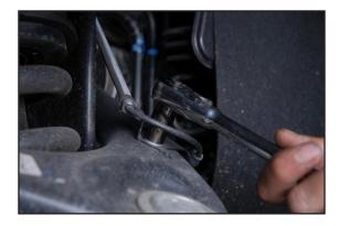
**3.** Remove the cotter pin from the upper ball joint and loosen nut with a 19mm socket.
