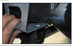
5. Using a 22mm socket, remove the lower shock mount bolt. The lower shock mount bolt may be difficult to remove so use an oil lubricant and a long punch to remove the bolt. Next remove the sway bar from lower A-arm by using a 19mm socket. As always be careful not to damage the bolt or the threads.
