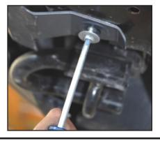
**9.** Slide the King coil over in bottom first then push up on upper a-arm. Slide the shock into the upper mount. Start the four 3/8 x1 inch bolts to hold the shock in place but don't tighten. Line up
