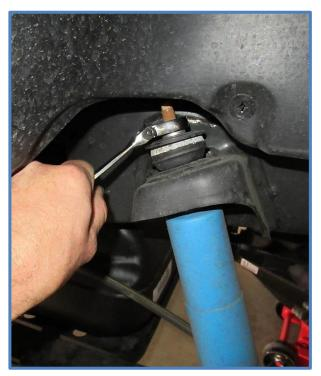
2. Remove the lower nut and bolt using a 17mm wrench and socket, then remove shocks.
