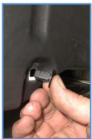
4. Pull fender liner back and install the reservoir bracket to the existing holes in the tabs hanging down from the steel bed using the supplied 1/4" bolts, nuts and washers.
