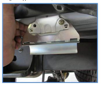
5. Tighten both mounting bolts using a 7/16 wrench and socket. Then let the plastic fender liner down and install the supplied push rivet into the hole.
