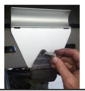
**4.** Remove the nut, washer, anodized blue retainer and upper rubber bushing from the King shock. Feed the shock up into the upper mount then replace the bushing, retainer, washer and nut on top of the pin as shown leaving the nut finger tight. Next insert the lower shock eye into the bottom mount and install the bolt, washer and nut finger tight.
