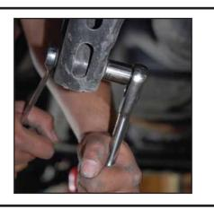
NOTE: The rubber bushings on your King Shocks are different from each other. Make sure the taller bushing is on the bottom next to the body of the shock as shown.
