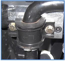
11. Install the skid plate tubular support pieces using the spacers and M10x30mm bolts provided in the kit.
