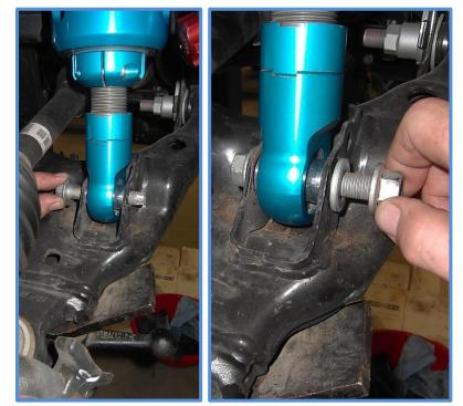
12. Jack up the lower control arm so the upper mounting plate is tight against the upper mount and install the 3/8 HD washers (CW1701) and 3/8 nuts (CN2711).
