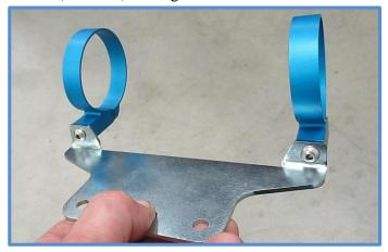
10. Install reservoir brackets. On the driver's side of the truck (left), remove the bolts holding the brake line bracket to the frame as shown. Insert the reservoir bracket between the brake bracket and the frame. Replace the bolts and tighten.
