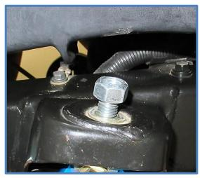
7. Place the rod end in the lower mount and install the 1/2 X 2-3/4" bolt (CB4730) with washer (CW1702). Be aware that these shocks have offset bearing spacers, the longer spacers should be towards the frame which offsets the shock out towards the wheel, this is to provide clearance between the shock and the leaf spring. Make sure the longer spacers are towards the frame. Install the washer (CW1702) and thin nylock nut (CN2800) and tighten both shock mount bolts to 90 ft-lbs.
