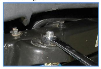
9. Next prepare the reservoir brackets for installation by attaching the reservoir clamps. Attach the clamps to the bracket as shown below using the supplied 1/4 X 1/2" BHCS (CB2420) and tighten with a 5/32 Allen wrench.
