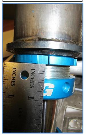
Thread the upper lock ring onto the cylinder and tighten both rings using a hammer and punch or screwdriver. Once the lock rings are tight, be sure to tighten the set screws.
