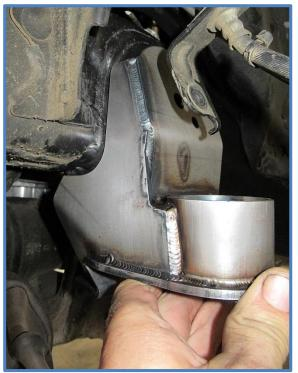
8. Once test fitting is complete, prep the vehicle for welding by removing the paint all the way around the front and sides of the modified factory bracket.
