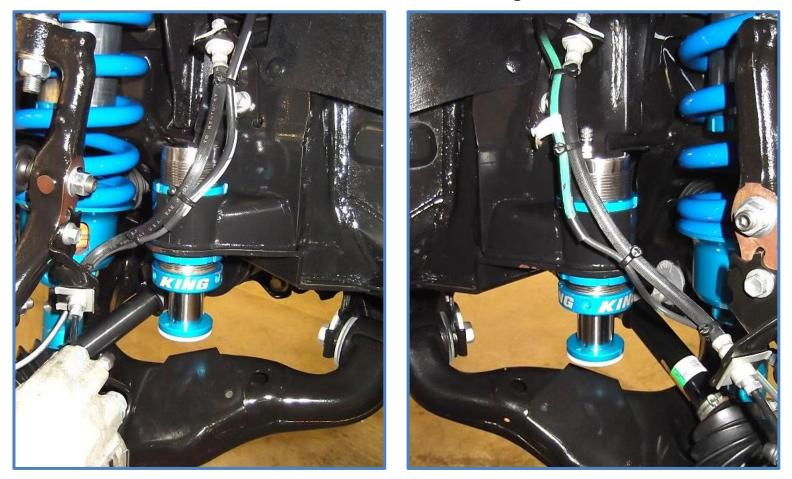
**DOUBLE CHECK ALL HARDWARE:** Reinstall shocks and any other components that were removed or disconnected during bump stop install. Make sure everything is installed correctly and all hardware is tight before reinstalling tires. Install tires, remove jack stands and lower vehicle to the ground. Recheck all hardware and lug nuts after 100 miles and periodically after that as part of routine maintenance.
