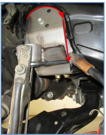
11. When welding is complete, prep and paint all bare metal to protect from rusting.
