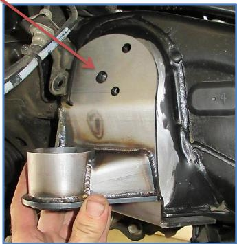
This kit **DOES** require welding. All welding must be performed by a professional welder. Do not weld on any shock or bump stop components. Welding near or on shocks may void the warranty and/or cause the product to fail. If any parts are missing, or for tech assistance; Contact King Off Road Racing Shocks: 714-530-8701 Most important after the install, Feel the difference and have fun.
