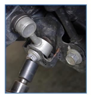
NOTE: To make sure sway bar does not make contact with the shocks, we recommend rounding off the corners of the sway bar as shown in the photo. Trim, grind and paint the sway bar ends while the shocks are removed.
