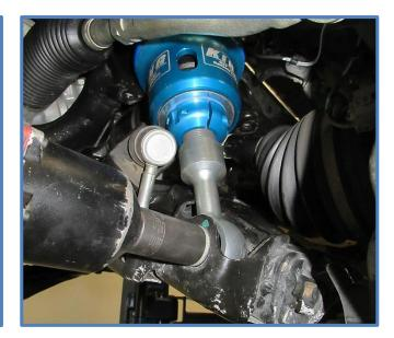
11. Connect upper control arm to the spindle following the instructions that came with your control arms. Then reconnect ABS and brake line brackets. The Total Chaos arms shown here provide a tab and hardware to mount the factory ABS line bracket to the new control arm.
