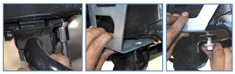
13. Slide two of the reservoir clamps onto the reservoir (see photo's for proper orientation). Position the reservoir over the reservoir bracket and install the 1/4 X 1/2" BHCS (CB2420). Use a 5/32 allen wrench to secure clamp to bracket. Then install the 1/4 X 1" SHCS (CB1501) to tighten clamp, center reservoir and adjust as needed. Tighten clamp using a 3/16 allen wrench. See step 16 for note on trimming plastic on right side.
