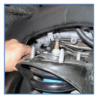
7. Install King Shocks. (Shocks are side specific) First place the shock into the upper mount and insert upper mounting studs into upper mount on vehicle. Photos below show the left side.
