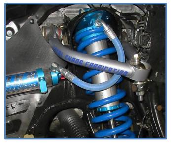
8. Place the rod end into the mount on the lower control arm, you may need help pushing down on lower arm while inserting rod end. Make sure the longer bearing spacer is facing forward.
