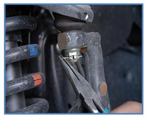
3. Remove sway bar bolt using a 19mm socket.
