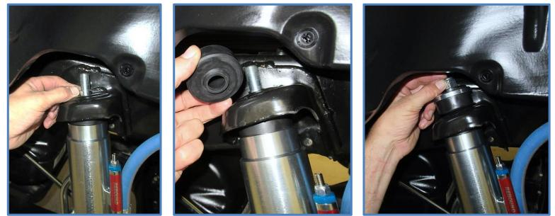
8. Tighten the upper nut using a 15/16 wrench. You should tighten the nut until the bushings start to compress, there should be about 1/8 – 1/4" of thread protruding past the nut. Do Not Overtighten!
