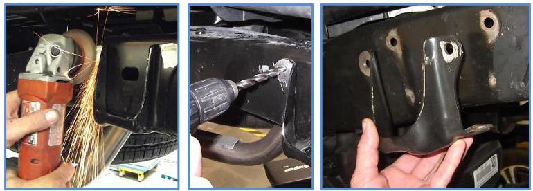
3. Place the bracket in position on the frame and install the 7/16 X 1" bolts (CB4601) with washers (CW1001). It may be necessary on some vehicles to enlarge one or more of the holes in the frame to install hardware. Tighten the lower bolts first using a 5/8 wrench and socket, then tighten the upper bolts.
