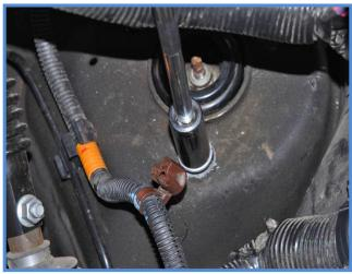
3. Loosen the nut for the ball joint on the upper control arm and separate control arm from upright but do not fully remove yet.
