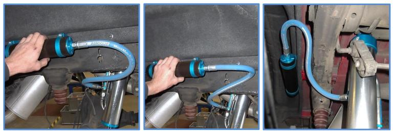
14. Once the reservoirs have been secured in the final position you can attach the KING nameplate. Be sure to clean the reservoir with alcohol. Peel the adhesive backing off the back side of name plate and place the plate on the reservoir. Use zip ties to hold the plate tight to the reservoir for at least 72 hours. Zip ties can be removed after 72 hours. (<u>3M recommends a 72 hour cure time for maximum bond strength</u>
