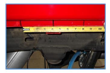
5. Find the center of the two outside lines and use a center punch to mark the location for drilling. Drill 1/4" holes.
