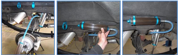
12. Install the  $1/4 \ge 1$  socket cap screws and snug so the reservoir can still be rotated in the clamps.
