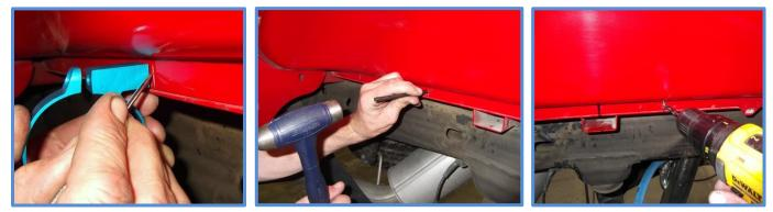
6. Place the fender liner back in position on the vehicle to mark for drilling but don't screw back in yet. Mark the two holes, remove from vehicle and drill 1/4" holes. Place the fender liner back on the vehicle, make sure the holes are lined up. Replace all the screws and tighten.
