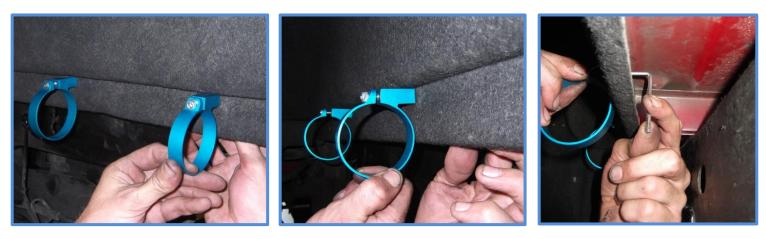
8. Place the reservoirs in the clamps. Starting with the left side, loop the reservoir into the clamps as shown.
