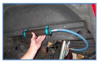
9. Use the provided loop strap, fender washers and 1/4 x 1" bolt with nut to hold the hose to the frame. (Left side only) Place loop strap on hose, place oval washer in the recessed oval hole in the frame. Use the 1/4 x 1" bolt and nut with fender washer on the back side of frame to attach hose. This step is important to make sure the hose does not rub on tire and leaf spring.
