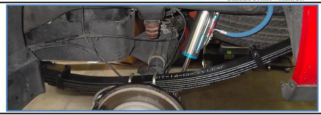
This leaf spring is designed to lift the rear 1"-  $1\frac{1}{2}$ " over stock without the factory lift block (if applicable). Install leaf springs without the block. Factory lift block can be added if a taller ride height is desired.
