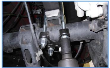
10. Raise the rear end up again and support frame rails with jack stands and let the suspension hang at full droop with the shocks installed, bolt the brake line brackets back in place (you may need to bend the brackets slightly so that the brake lines are not tight at full droop). Place ABS lines back in clips, you may need to pull some slack for the ABS lines so they aren't tight at full droop.
