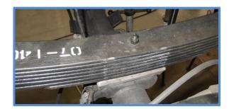
9. With the new leaf springs installed, place the tires back on the vehicle and lower vehicle to the ground. Tighten all leaf spring bolts (main mounting bolts, shackle bolts and U-bolts) only when the vehicle is sitting on all fours at ride height with the weight of the vehicle on the suspension.
