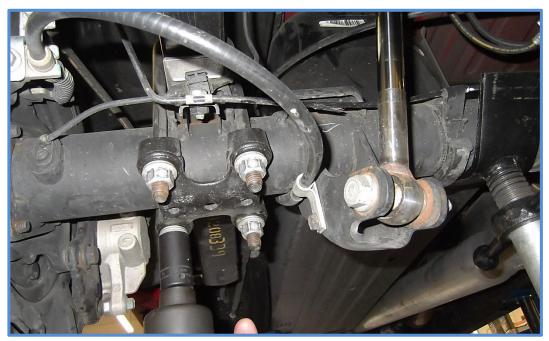
3. Remove the nuts from the leaf spring mounting bolts. Hold the end of the front bolt with a 12mm wrench and loosen the nut with a 24mm wrench. Hold the end of the rear bolt with a 10mm wrench and loosen the nut with a 21mm wrench. Also, loosen the shackle nuts slightly so the shackle will swing down easier for removing the spring bolt.
