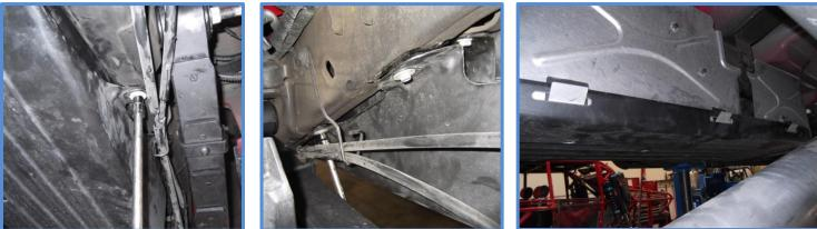
5. Place supports under the gas tank and remove the bolts holding the straps and remove straps. Lift the vehicle slightly or lower the tank and inch or so. You should now be able to move the gas tank over enough to get the bolt out... it's tight in there but it can be done.
