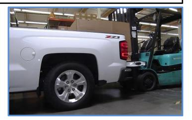
8. With the suspension bottomed out, check for clearance issues. On the left side make sure the bump stop has clearance between the bump stop and the strike pad. Also on the left side make sure the lower strike pad does not contact the gas tank. Make any necessary adjustments. On the right side make sure the bump stop has clearance between bump stop and the strike pad. Make any necessary adjustments at this time.
