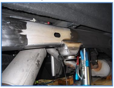
4. Next prepare your axle for welding. Grind the paint from the existing bump pad on the axle and the shock mount area as shown below.
