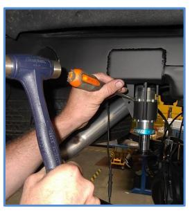
Tighten set screws when final position has been determined
