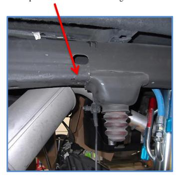
2. Remove factory bump stops using a 10mm socket to remove the bolt located inside the foam bump.
