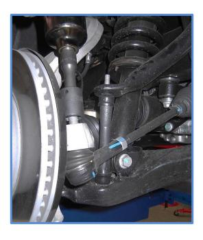
6. Remove the bolt from the lower shock mount using a 21mm socket. (Nut is welded)
