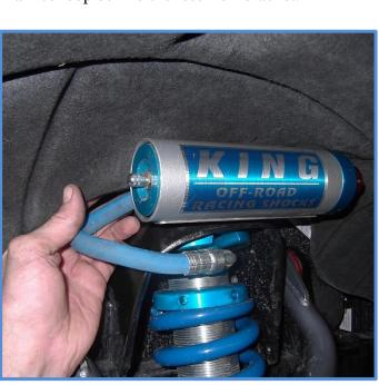
12. Twist the reservoir up so the hose is out of the way, line up the mounting holes and install the supplied 3/8" x 1" bolts. Start all the bolts by hand then jack up the lower control arm until the shock is tight against the upper mount. Use a 9/16" ratchet wrench to tighten the upper bolts.
