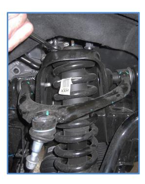
through the a-arm first then place the shock in position on the vehicle. Shocks are side specific... See Photo's.
