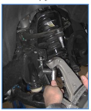
4. Remove the nut from the tie rod end using a 21mm socket and separate the tie rod end from the knuckle.
