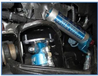
3. Place the reservoir mount onto the studs on top of the factory shock mount. Place the supplied 10mm washer on the stud followed by the 10mm nut provided in the kit. Tighten nuts to 35 ft lbs.
