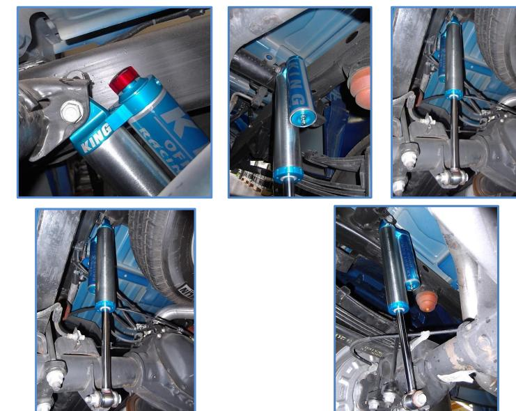
**DRIVERS SIDE:** View of left side looking towards front of truck. Make sure the reservoir is facing the front of the truck. It will be directly above the axle housing.
