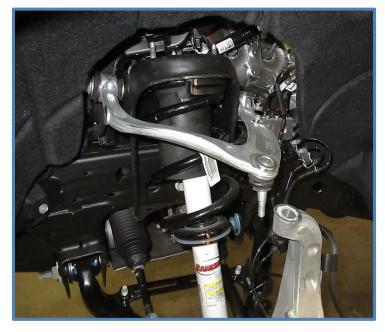
5. Remove nut from tie rod end using a 21mm wrench or socket and separate tie rod end from knuckle.
