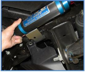
18. Using the factory bolt you just removed and the 90° nut plate provided in the kit, secure the reservoir bracket to the frame. The reservoir bracket will sit against the frame and the plastic piece will go over the reservoir bracket as shown. Install the factory bolt and tighten.
