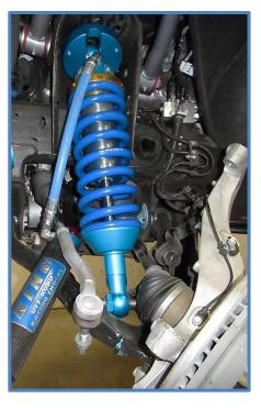
9. Install the provided 3/8 x 1" bolts (CB4701) with HD washers (CW1701) in the upper mount and tighten to 35 ft. lbs.
