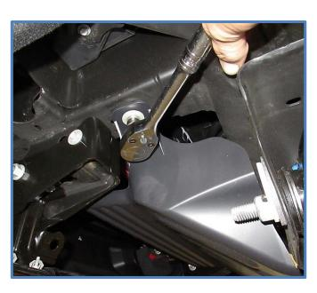
15. Remove the clip in the frame that the bolt was attached to. The reservoir bracket will mount to frame using this hole.
