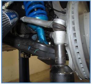
13. Reconnect ABS lines and brackets. Re-clip the lines into their holders and reinstall the bracket on left side.
