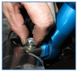
11. Reconnect upper control arm to knuckle and tighten hardware.
