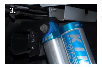
Reinstall the new KING shock by aligning the top shock mount and installing the bolt and nut. Do the same process on the lower shock mount.
