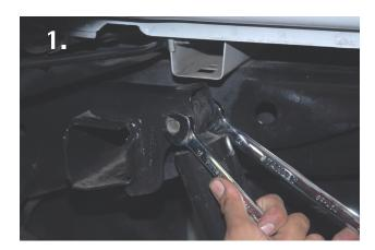
With the vehicle safely supported with jack stands start by removing the upper shock mount bolt using a 15mm wrench on the bolt and a 18mm socket or wrench on the nut.
