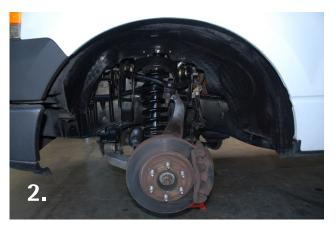
With the vehicle level on the ground set the emergency brake and block the rear tires. Using a floor jack, raise the front end and support the frame rails with jack stands for safety. Then remove the front tires. NOTE: Never work under an unsupported vehicle.
