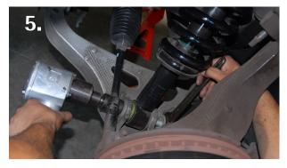
Remove the lower shock mount bolt /nut using a 27mm socket and a 30mm end wrench. With all hardware removed pull down on the stock coil over and remove from A-arm assembly. NOTE: This can be difficult for one person because of the close proximity of the ball joint arm. You may need a second person to help hold the ball joint assembly to one side as you remove the stock coil over.
