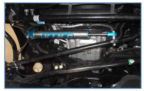
Double check your install, make sure the stabilizer is mounted properly and all hardware is tight. Recheck the hardware after 50 miles and periodically after that as part of routine maintenance.
