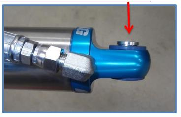
3. Install your new King Shocks with the reservoirs facing away from the axle as shown on next page. The driver's side (Left) reservoir faces towards the rear of the vehicle, the passenger side (Right) reservoir will face forward. Push the shock onto the top mounting stud with the longer spacer towards the frame and thread the factory nut on but do not tighten.
