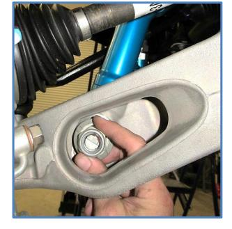
12. Reconnect upper control arms to spindle and tighten to factory specs.
