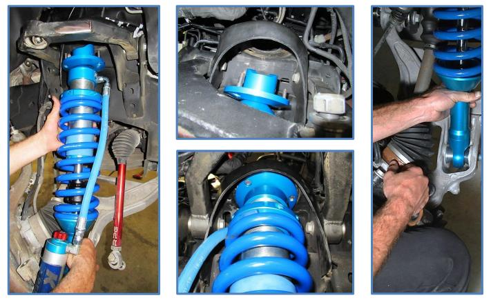
10. Place the HD 3/8" washers (CW1701) on the upper mounting studs followed by the 3/8" Nylock nuts (CN2711). Tighten nuts to 35ft-lbs.
