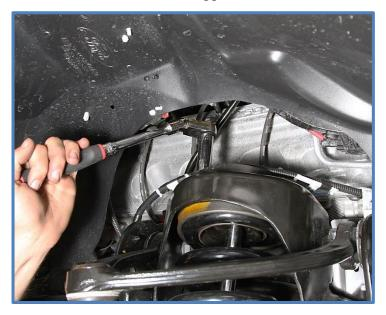
8. Remove the factory shock from the vehicle as shown.
