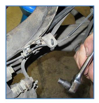
16. Install reservoir brackets to the bottom of the frame using the skid plate bolt and bracket. Unbolt the skid plate and bracket and install reservoir brackets as shown below.
