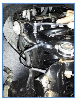
3. Remove cotter pin from upper A-arm ball joint stud then remove nut and separate upper A-arm from spindle.
