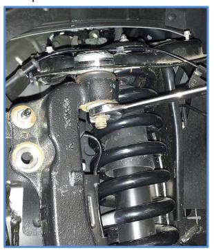
4. Remove the lower shock mount bolt.
