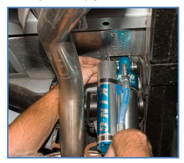
5. Place the rod end in the lower shock mount and install the factory bolt. Tighten lower mounting bolts to factory specs.
