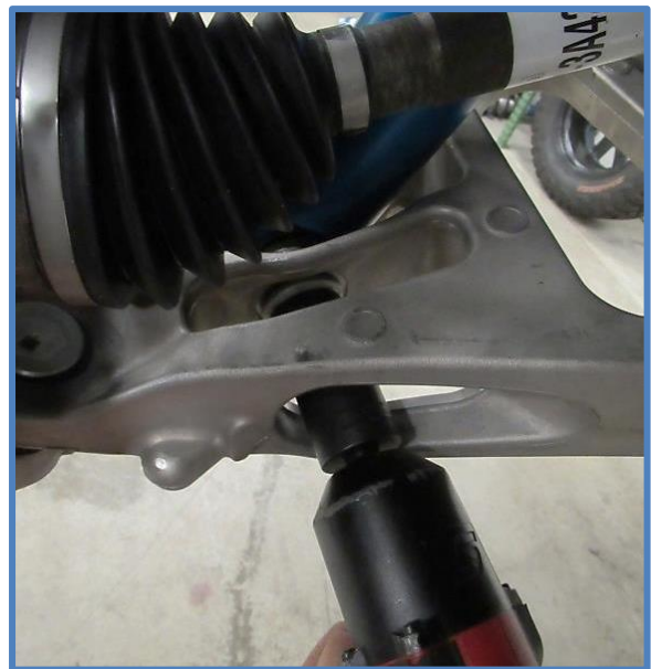
Lower Mounting Bolt – 400 ft-lbs
