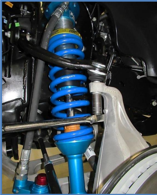
Upper Ball Joint Nut – 85 ft-lbs
