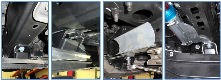
**NOTE: 2wd** – For 2wd models and/or vehicles without tow hooks you may need to remove bumper to install reservoir brackets if access to mounting points is not available. Use the supplied 10mm hardware to attach brackets to existing holes in frame if tow hooks and tow hook hardware are not installed on your vehicle.
