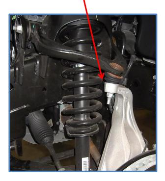
5. Using a 15mm socket, remove the three nuts from the top of the shock assembly and remove the shock.
