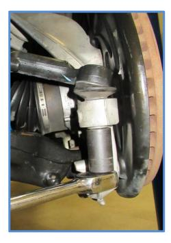
4. Remove the nuts from the lower shock mount using an 18mm socket. Save the nuts you will reuse them to mount the King Shocks. 3. Disconnect the upper A-arm from the upright. Using a 21mm socket, loosen the nut on the A-arm ball joint. Separate the ball joint from the upright using proper ball joint tools.
