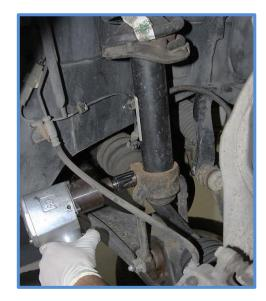
6. Remove the clevis from the factory shock. This will usually require using a large hammer. You will be reusing the clevis so be careful not to damage this piece when removing.
