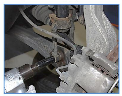
4. Remove the bolt from the strut fork Clevis at the bottom of the shock body using a 21mm socket.
