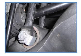
13. Now with the floor jack still under the lower control arm raise the jack until the weight of the vehicle is on the suspension and the frame just starts to lift off of the jack stand. With the weight of the vehicle on the suspension you can tighten all hardware, start with the 4 upper bolts, then tighten the clevis/strut fork bolt and finally the lower mounting bolt.
