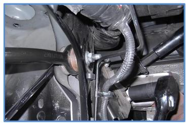
9. Install the reservoir brackets using the upper A-arm and brake line bracket bolt locations to mount the reservoir brackets as pictured below. Reuse original hardware and tighten.
