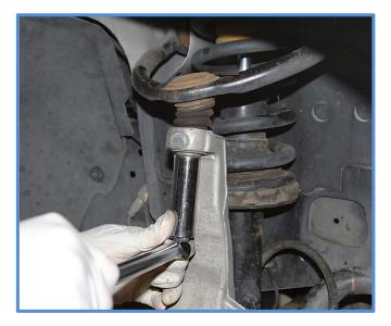
5. Remove the nut from the lower mounting bolt using a 24mm socket. After removing the bolt you can lower the jack so the shock is free hanging and clear of the lower control arm. Pay attention to the ABS and brake lines as you do this to ensure the lower control arm and steering knuckle are not hanging by these lines.
