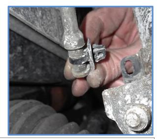
**Helpful Hint:** Keep a floor jack under the lower control arm on the side you are working on, this will come in handy for moving the suspension up and down to remove and install parts.
