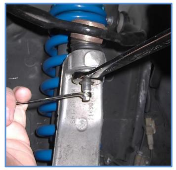
16. Insert the ABS sensor wire clip into the slot on the ABS line bracket as shown in photo.
