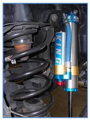
Make sure everything is installed correctly and all hardware is tight before reinstalling tires. Install tires, remove jack stands and lower vehicle to the ground. Recheck all hardware and lug nuts after 100 miles and periodically after that as part of routine maintenance.
