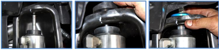
3. Install factory nut and bolt for lower mount and tighten. Jack up the axle so that the shock is tight against the upper mount and tighten nut so that the bushing just starts to compress, do not overtighten nuts.
