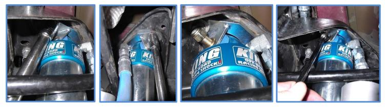
4. Put the rod end into the lower shock mount, insert the bolt, install nut and tighten.
