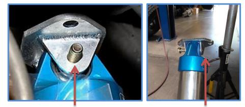
3. To make installation easier, remove the nut from the top mount as shown above. You can slide the bolt over to gain access to the factory mounting bolts above it. Insert the shock assembly into the frame pockets, Install the factory mounting bolts and tighten. After the mounting bolts are tightened install the nut and washer to the through bolt on shock and tighten.
