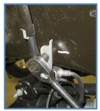
4. With the shocks removed and sway bars disconnected you can lower the axle and remove springs. Pay attention to the brake/ABS lines, wiring, breather tube, etc. when lowering axle and removing springs.
