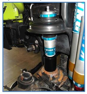
6. Once the bump stop position has been determined, tighten the locking nuts/collars and set screws.
