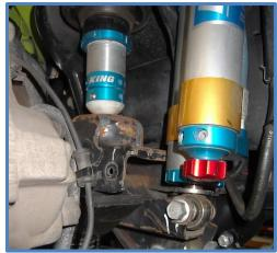
14. With the bump stops properly adjusted you can now tighten the nuts and set screws. Use a punch and hammer to gently tap the nuts until they are tight. Now apply locktite to the set screws and tighten.
