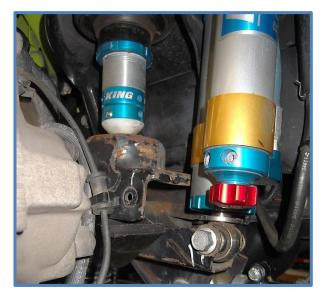
3. When installing the spacers provided with the King Bump Stop Kit, center the spacer on the axle's spring mount and use a 1/4" center punch to mark the holes.
