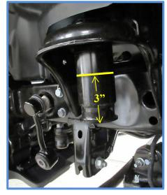
8. Use a sawzall or cut off wheel to make a nice straight cut on the line.
