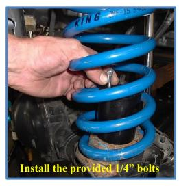
8. Install bolts, washers, nuts and tighten.
