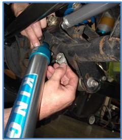
6. Install steering stabilizer on tie rod bracket. Install 3/4" spacer first, then steering stabilizer followed by the small spacer and nut. Tighten nut with 18mm wrench/socket.
