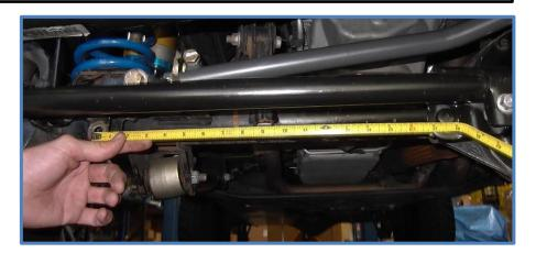
5. Install steering stabilizer on axle end first with 3/8" bearing spacers, tighten bolt with 18mm wrench/socket. Photos below show the steering stabilizer mounted to the axle bracket.
