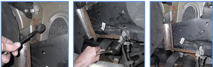
9. The King Shocks are side specific, be sure the shocks are being mounted on the correct side. (The hose should be towards the front of vehicle) Having someone hold the shock in position while someone else is starting the upper mounting bolts is the easiest way to install the coilover. Get the upper mounting bolts started to hold the shock in place first but don't fully tighten yet.
