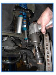
14. Place reservoir in the cradle and install hose clamps, position reservoir so the hose does not contact upper control arm.
