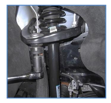
6. Remove the three nuts on the upper end of shock using a 13mm socket. These are located inside the engine compartment. Be aware that the shock is now hanging by the studs on the upper mount. Be prepared to hold the shock while removing the final nut or have someone hold it for you so it does not fall and cause injury or damage to vehicles components.
