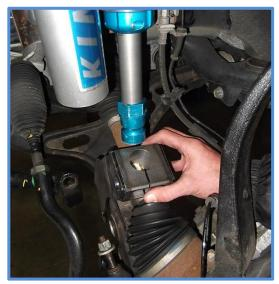
11. Attach Clevis to the lower control arm using the factory bolt but do not tighten yet.
