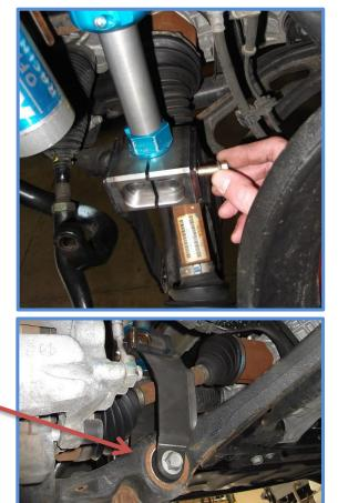
12. With all of the hardware installed but not tightened yet, jack up the lower control arm so that the weight of the vehicle is on the suspension to the point where the frame is coming off of the jack stands. Now you can tighten the **three upper mounting bolts**, the **clevis pinch bolt** and the **lower OE shock mounting bolt**.
