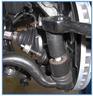
5. Remove the lower shock mount bolt using a 21mm socket on the bolt head and a 24mm wrench on the nut.
