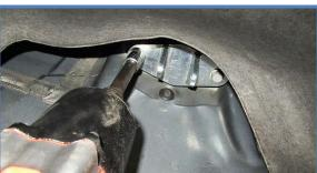
4. Place shock in position so that the reservoir is towards the rear of the vehicle and install the 1/2" x 2.75" bolts (CB4730) with washers (CW1702) and nuts (CN2801) in the upper mount first. **Torque bolts to 110 ft/lbs** using a 3/4 wrench/socket.
