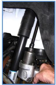
Remove the two lower push pins holding the fender liner to gain access to the upper mount when installing the King Shocks.
