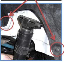
3. Install King Shocks by first installing the upper mounting brackets using the factory bolts. Remove upper mounting brackets (25035-102) from the shocks and install on vehicle first.
