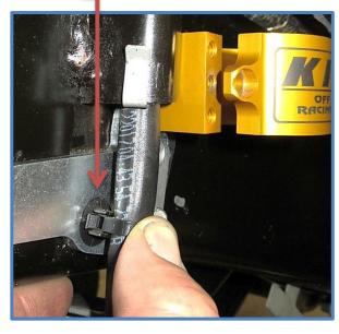
7. Now use the bent threaded nut plate included in the kit to secure the reservoir bracket on the other end. Place the nut plate in the large hole in the frame and line up with the hole in the reservoir bracket. Use the 1/4 X 1" bolts (CB4502 with washer CW1501) to thread into the nut plate.
