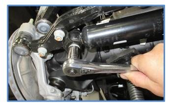
3. Place the King Steering Stabilizer on the vehicle as shown using the factory hardware.
