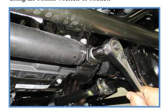
2. Remove the nut from the bracket on the tie rod using an 18mm wrench or socket and remove bolt.
