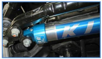
5. Install factory hardware on the axle end and tighten to factory specs.
