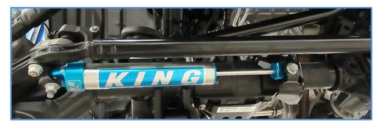
Double check your install, make sure the stabilizer is mounted properly and all hardware is tight. Recheck the hardware after 50 miles and periodically after that as part of routine maintenance.
