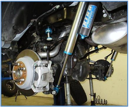
Photo below shows the suspension bottomed out with shocks installed and bump stops properly adjusted.
