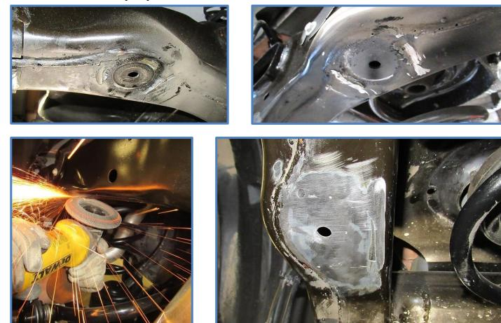
5. Use the template provided in the kit to mark the center of the hole for the hole saw. Hold the template against the inside edge of the frame as shown. Line up the slotted hole in the template with the existing hole in the frame. Use a punch in the small hole next to the slotted hole in the template to mark the center for the hole saw.
