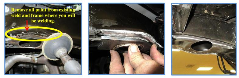
10. Prep work area for welding. Protect the surrounding area from weld splatter. Pay special attention to fuel lines, fuel tank, wiring, brake lines, brakes, etc.
