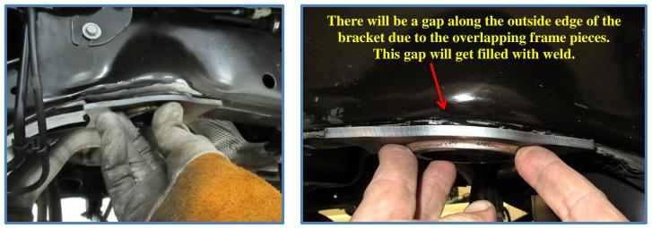
The short flat sections on the back side of the bracket will line up with the radius on the inside edge of the frame. The center section will stick out past the inside edge and does not get welded.
