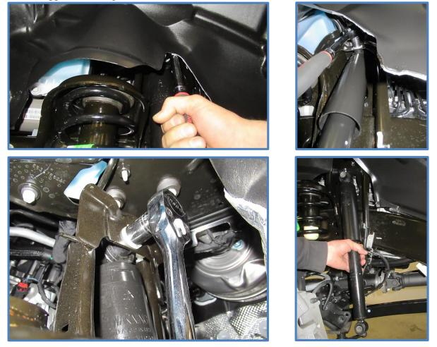
3. Install the King shocks using the factory hardware. Place the shock in the upper mount with the longer spacer facing in towards the frame. Insert the factory bolt and tighten to factory specs. Install shocks with cylinder on top and shaft mounted to the axle as shown.
