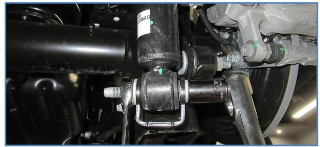
3. Remove upper bolt using an 18mm wrench or socket and remove shock.
