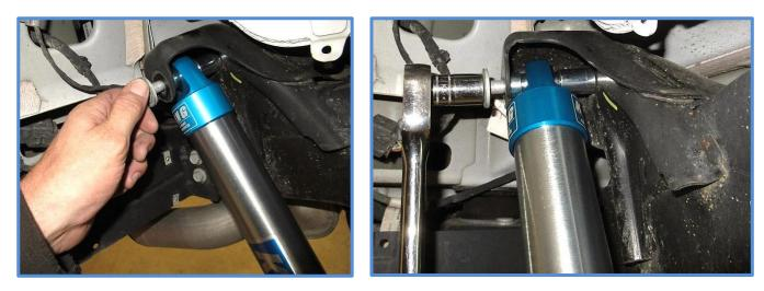
5. Place the rod end in the lower mount and install the factory bolt and nut. Tighten to factory specs.
