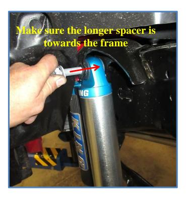
5. Place the rod end in the lower mount, install the factory hardware and tighten to factory specs.
