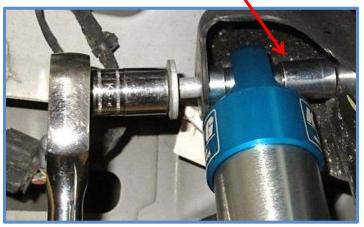
4. Place the rod end in the lower mount, install the factory hardware and tighten to factory specs.
